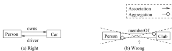
Figure 3. Aggregation integrity constraint.
